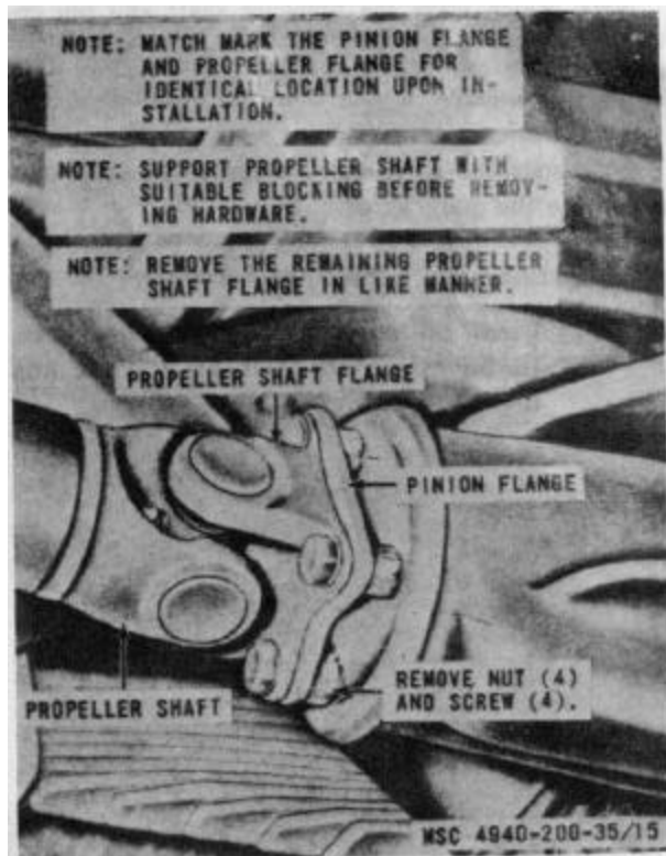
Figure 15. Propeller shaft, removal and installation.
